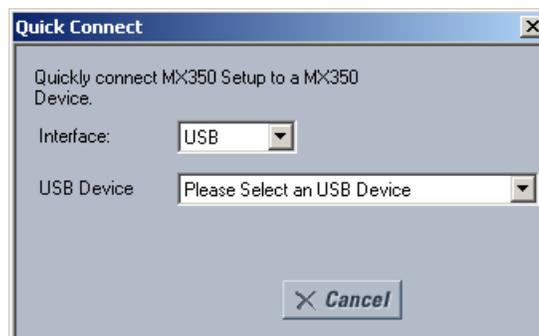
As indicated by the window, the "Quick Connect" feature can quickly connect the software to a front port if the USB is selected in the interface drop-down list. Select "Relay" and press the **Connect** button.
